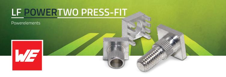
**LF PowerTwo Press-fit** Powerelements are two-piece lead-free high current contacts and a solution patented by Würth Elektronik ICS for the screw technology on PCBs. They enable a permanent and reliable connection or mounting on the PCB without adding stress. Depending on the pin arrangement and the corresponding layout, currents of up to 500 amperes are possible.
