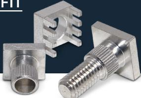
**PowerTwo Press-fit** Powerelements are two-piece high current contacts and a solution patented by Würth Elektronik ICS for the screw technology on PCBs. They enable a permanent and reliable connection or mounting on the PCB without adding stress. Depending on the pin arrangement and the corresponding layout, currents of up to 500 amperes are possible. The assembly method allows individual adjustments regarding dimensions.
